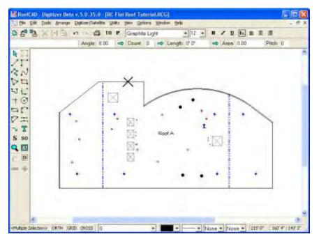
Anytime you add an object close to the edge of the roof you need to be careful not to miss putting the object on the roof. This is because of the way RoofCAD determines what roof an object belongs to. When you add something to the drawing, RoofCAD determines which roof the object belongs to by calculating if the object is within the perimeter of the roof. This means the object must be directly on a perimeter line or within the perimeter (i.e. on the roof). So as you can imagine. When you place a
