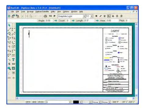
Templates are just normal RoofCAD files that have been set up to help you start drawing faster. You can modify the templates shipped with RoofCAD or create new ones.
