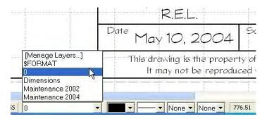
This is a list of the layers in this drawing. The 0 layer is where we drew the roof plan. The \$FORMAT layer is where the legend and title block are stored. The two Maintenance layers are there as an example of where you could record annual maintenance information. The Dimensions layer is where the dimension lines are stored.
