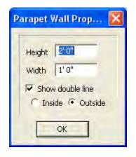
Notice that you can change the height and width of the wall as well as tell the system whether to draw the parapet as a double line. The inside and outside option tells the system where the second line is to be placed, either inside or outside of the existing line.
