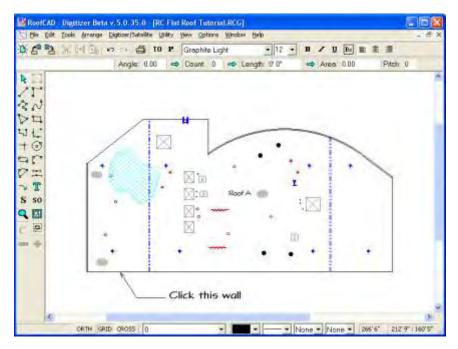
• Move the mouse pointer below the wall and click again. The wall is now dimensioned like the following illustration:
