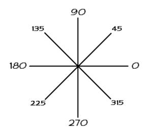
Angles in RoofCAD work the same as any CAD program. When you draw a line the angle of the line is relative to the starting point. Reference the above diagram when deciding the number to input for an angle. If you think of the preceding illustration as 8 separate lines that start from the center point you can see the angle you would have to enter for each line to run the direction that it does. The angles we display in the diagram are the angles you would use for 90 & 45 degree lines.
