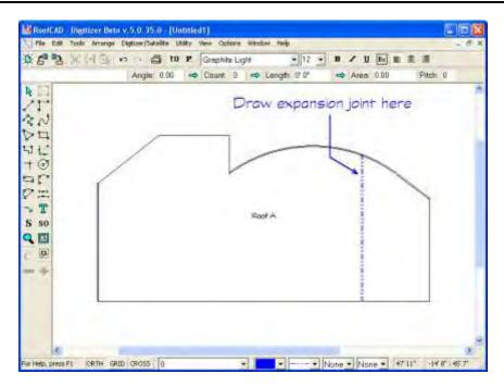
This is how you draw an expansion joint free hand. If you want to be more accurate in the placement of expansion joints or any other object you can use the keyboard.
