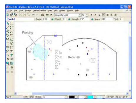
To draw this ponding area we clicked the mouse once at each of the points where the perimeter changed direction. To tell RoofCAD when you are finished drawing the ponding area, right click the mouse. You may have to try this a couple of times to get the hang of it. Go ahead and try drawing the Ponding area now.
